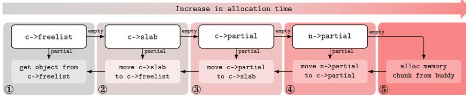
Figure 2: SLUB allocation of an object, where the terms `c` and `n` refer to the `kmem_cache_cpu` and `kmem_cache_node`, respectively. The free lists (i.e., `c->freelist` and `c->slab->freelist`) and slab lists (i.e., `c->partial` and `n->partial`) are checked to be either empty or partial.
