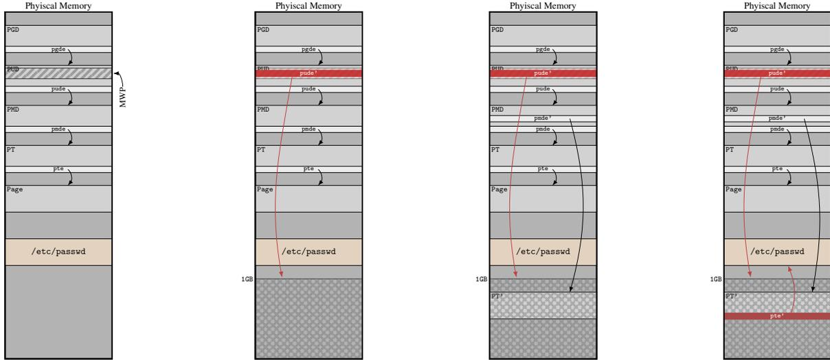
(a) SLUBStick has an MWP to a PUD page used for a user address translation. It aims to tamper with the targeted page containing data of `/etc/passwd`.
