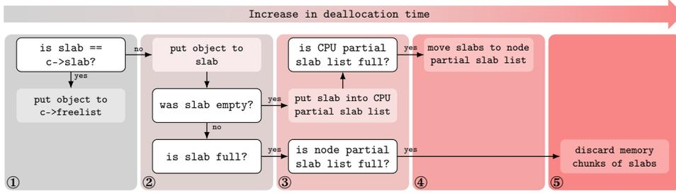
Figure 3: SLUB deallocation of an object, where the term `slab` refers to the slab that contains the object to be freed. The term `c` represents the `kmem_cache_cpu` associated with this slab. The `slab` is either active (i.e., `slab` stored as `c->slab`), or stored in the partial slab list (i.e., `slab` located within `c->partial`) or node partial slab list (i.e., `slab` located within `n->partial`).
