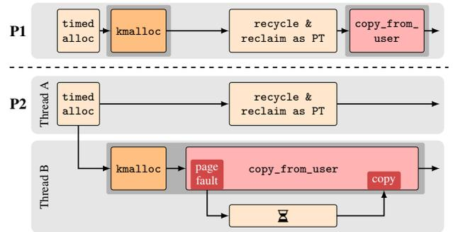
Figure 7: The execution timeline of persistent code patterns 1 (P1) and 2 (P2), where `timed alloc` performs persistent allocations combined with our timing side channel. `kmalloc` allocates the memory slot referenced by the dangling pointer. Since this slot resides on the page table after recycling and reclamation, `copy_from_user` overwrites page table entries.
