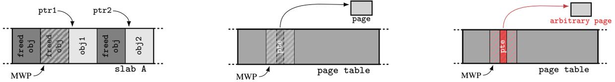
(a) *Stage 1* deallocates objects `obj 1` and `obj 2` to trigger the recycling process of `slab A`'s memory chunk, with a Memory Write Primitive (MWP) referring to it.
